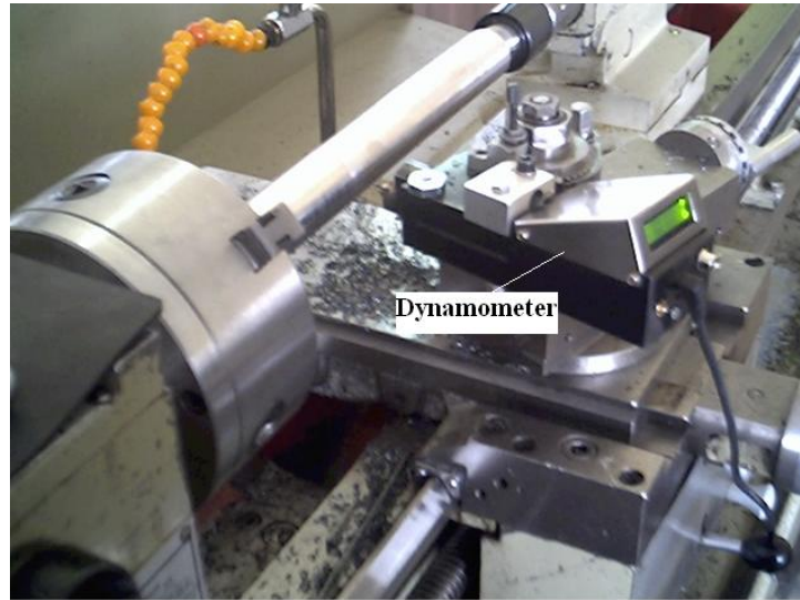
Fig. 2 Experimental view of cutting force registering in turning process
