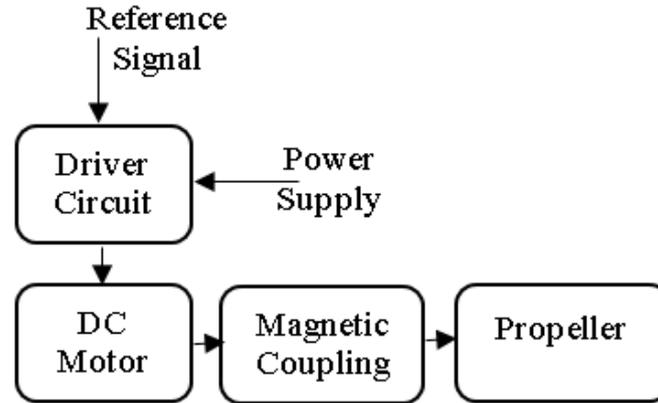
Figure 3. System Architecture
