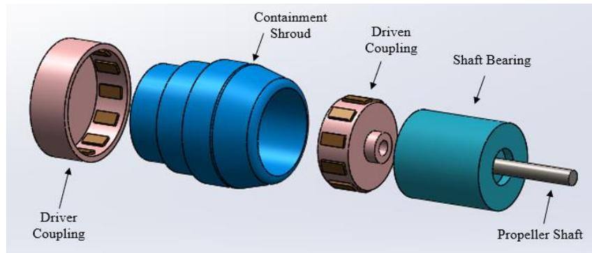
Figure 6. Magnetic Coupling
