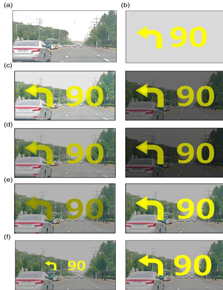
Figure 3. The types of the different factors influencing legibility. (a) Background photo. (b) Contents of the transparent on-screen display. (c) Recognized photo in terms of illuminance alter. (d) Recognized photo in terms of transmittance change. (e) Recognized photo in terms of max luminance alter. (f) Recognized photo in terms of font size alter. [Reproduced from reference 7 with permission. Copyright 2019, Journal of Information Display].
