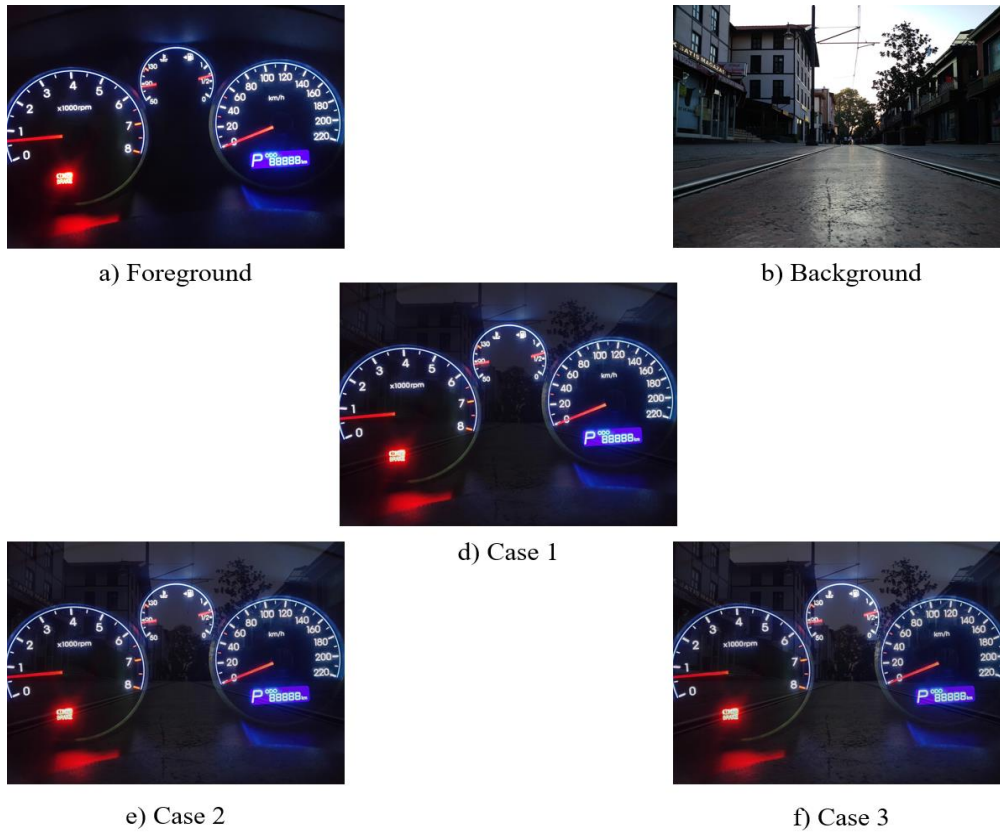
Figure 9. Some various cases. (d) Low transparency case with high foreground contrast. (e) Low transparency case with less foreground contrast. (f) High transparency case.
