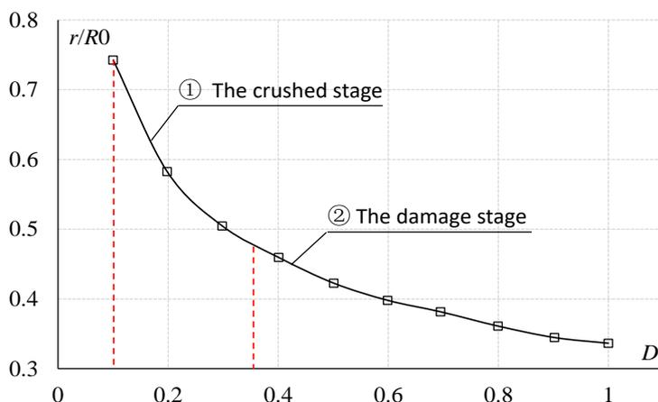
Figure 5. The relationship between fragment dimension and damage state
