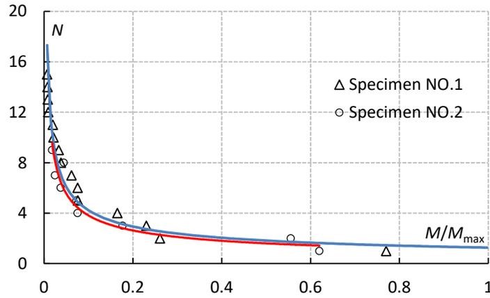
Figure 4. The quality-frequency distribution of red sandstone fragments
