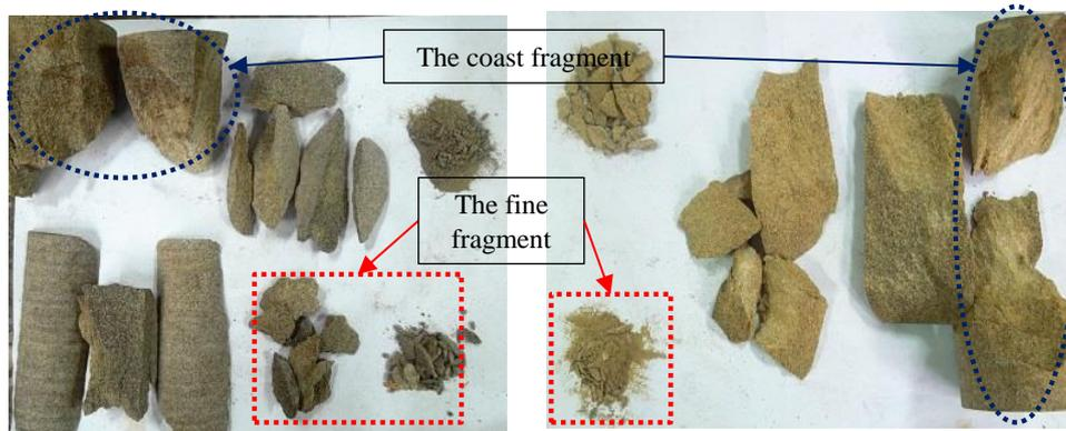
Figure 3. Rock fragments of red sandstone after UCT
