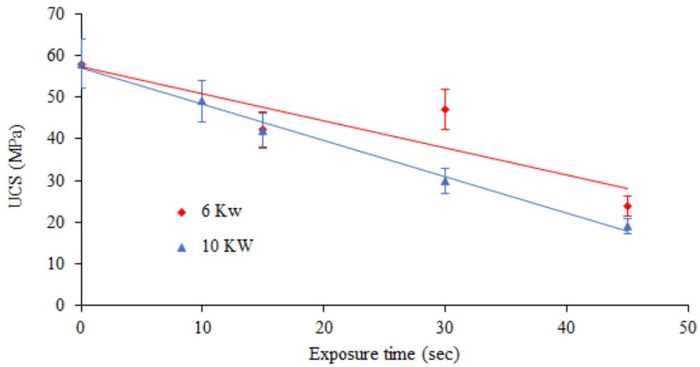
Figure 4. Unconfined Compressive Strength vs. exposure time at two MW power levels for TK
