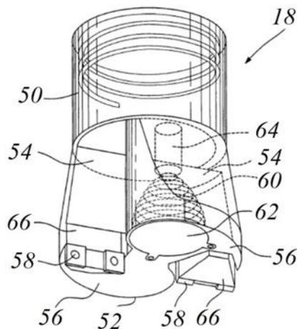
Figure 1. Conceptual design of a drag bit at McGill University equipped with microwave antenna. 18- Excavation bit; 50- Base body; 52- Cutting surface; 54- Sections; 56- Two wings; 58- Cutting tool; 60- Housing; 62- Cover plate; 64- Opening; 66- cutting tool holders [13, 14].
