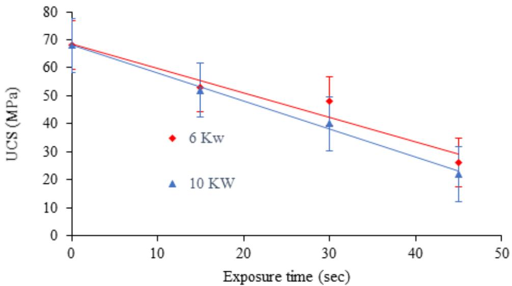
Figure 5. Unconfined Compressive Strength vs. exposure time at two MW power levels for limestone
