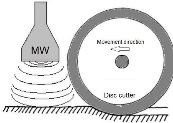
Figure 2. The schematic illustration of a microwave-assisted disc cutter [5, 14, 16]
