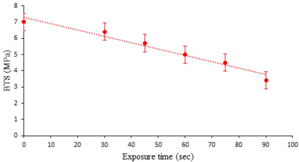
Figure 6. Brazilian Tensile Strength vs. exposure time at 3 kW MW power for TK
