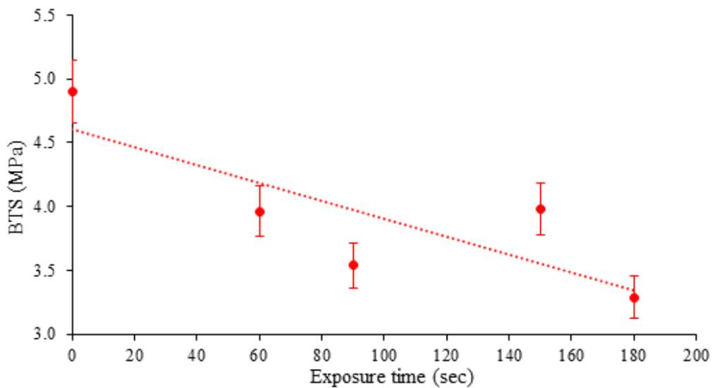
Figure 7. Brazilian Tensile Strength vs. exposure time at 3 kW microwave power for limestone
