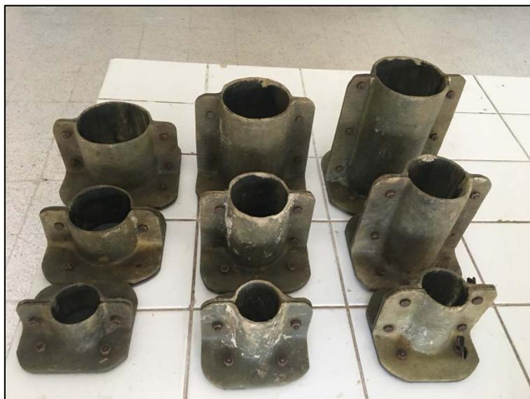
Figure 3. Molds specifically designed for bond tests.
